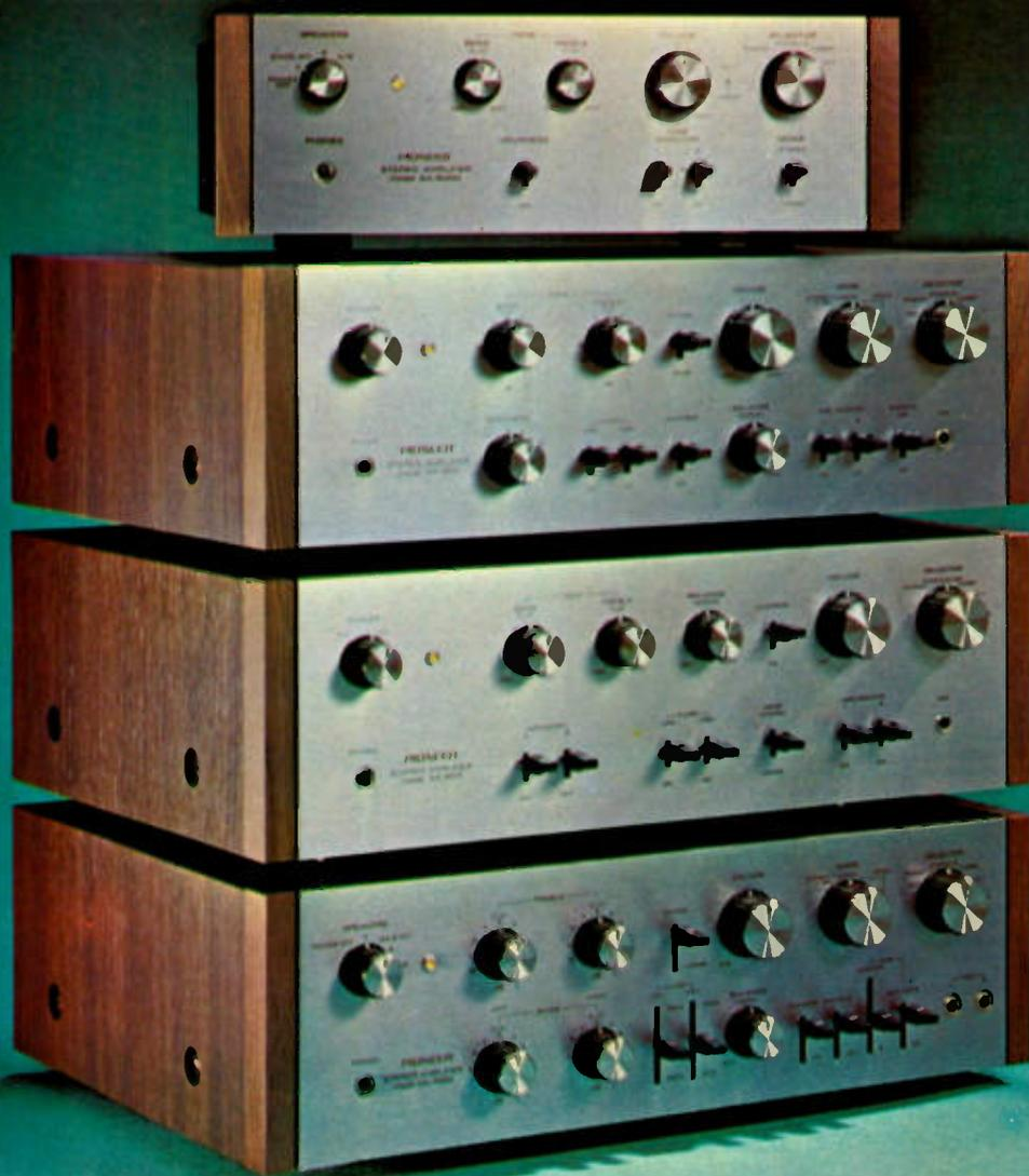
**SA-500A.** Continuous power output 10W per channel (both channels driven at  $8\Omega$ ). IHF power bandwidth 20-40,000Hz. Click-stop bass and treble controls; mode switch, loudness switch. Simultaneously drives two turntables or two decks (open reel, cassette, 8-track cartridge), two pairs of speaker systems.
